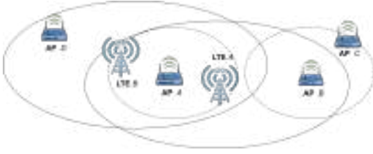
Fig. 2: Coexistence between LTE and Wi-Fi. Wi-Fi and LTE stations have different interference ranges.
