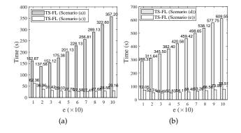
Fig. 11. Required time consumption for training a model with target loss  $(\pi=0.0132)$  under different local epoch numbers e and a fixed minibatch size n=500 based on (a) handwritten digit dataset and (b) traffic dataset.
