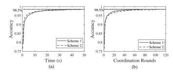
Fig. 1. (a) Model accuracy vs. training time, and (b) model accuracy vs. number of coordination rounds under two FL model training schemes: Scheme~1~(200~local~epoch~number,~20~mini-batch~size) and Scheme~2~(200~local~epoch~number,~10~mini-batch~size). The target accuracy of the trained model is set to 98.5%.
