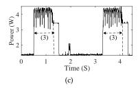
Fig. 6. (a) Recorded power tracking traces of an edge server (Raspberry Pi 4B) with four highlighted steps in each round of model coordination: (1) model distribution, (2) data uploading, (3) local model training, and (4) model uploading. (b) Comparison of time duration in step (3) under training parameters (e=10, n=3000), and (c) (e=10, n=1000).
