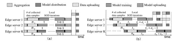
Fig. 2. Illustration of collaborative model training in an FEI system under: (a) synchronous coordination, and (b) asynchronous coordination.
