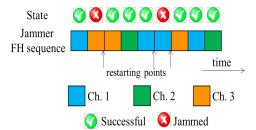
Fig. 6: Smart sweep jammer.
