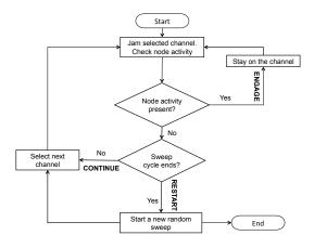
Fig. 5: **IBFD Reactive Sweep Jammer:** In each time slot, the jammer attacks currently selected channel and observes channel activity. If activity is observed, it stays on the channel and continuously attack it (ENGAGE). Otherwise, it RESTARTs a new sweep patten if the current cycle ends, else attacks next channel in the sweep cycle (CONTINUE).
