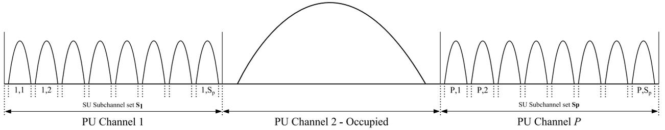
Fig. 1. PU channels and SU subchannels.
