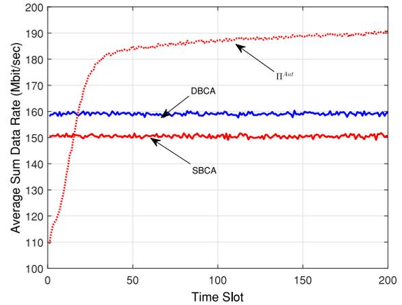
Fig. 6. Average sum data rate vs. time for the proposed  $\pi^{Aut}$  method, SBCA and DBCA, where  $|\mathcal{S}_p| = 8$ ,  $N_R = 50$  m, and  $I = 8$  users, with maximum CB capability of bonding 3 subchannels.
