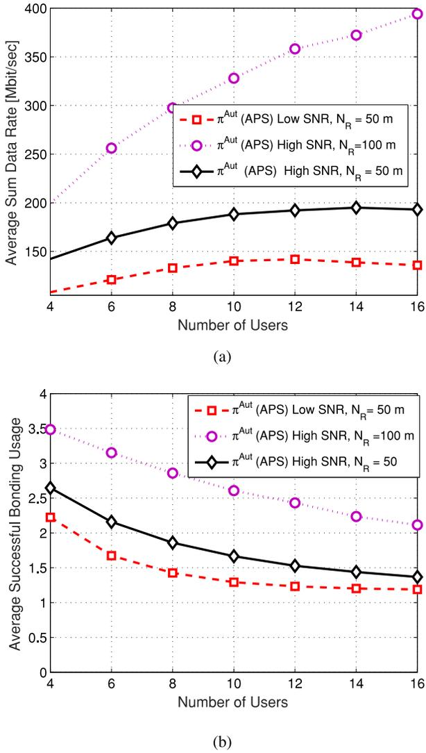
Fig. 8. a) Average sum data rate achieved and b) Average successful CB utilized under the  $\pi^{Aut}$  with APS CB selections for  $|S_p| = 8$ . Each user is with the same maximum CB capability which means that each user has the ability to bond all the subchannels.
