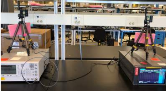
Fig. 6. Test setup with 4 \times 4 UPAs at the Tx and the Rx, signal generator and vector signal analyzer (operating on the 29 GHz band).
