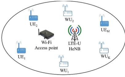
Fig. 1. System model for an LTE-U small cell, that is composed of an HeNB and  $M$  UEs, coexists with a Wi-Fi network, that is composed of a Wi-Fi AP and  $K$  WUs.
